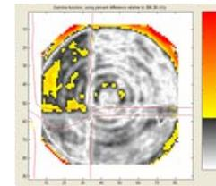
Fig. 5 Gamma index comparison (5% or 3 mm) between gel and unmodulated treatment plan. 88% of the pixels pass the gamma comparison.
