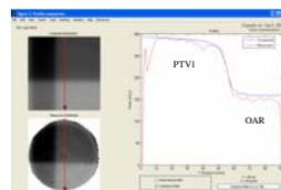
Fig. 4 Profiles through PTV1 and the OAR from gel measurements (red) and the unmodulated treatment plan (blue).
