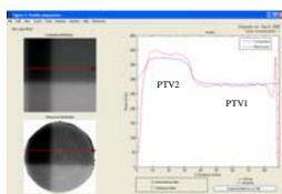
Fig. 3 Profiles through PTV2 and PTV1 from gel measurements (red) and the unmodulated treatment plan (blue).
