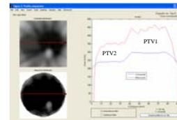
Fig. 6 Profiles through PTV2 and PTV1 from absolute gel measurements (red) and the IMRT treatment plan (blue). These look reversed from plan - confusing?
