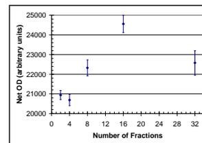
Fig. 9 Net OD for dosimeters irradiated to 3 Gy using a different number of fractions. Error bars represent one standard deviation.
