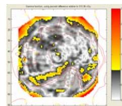
Fig. 8 Gamma index comparison (5% or 3 mm) between gel and IMRT treatment plan. 84% of the pixels pass the gamma comparison.
